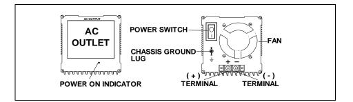
CAUTION: DO NOT REVERSE INPUT. USE RED BATTERY CORD TO CONNECT (+) OF A DC BATTERY TO (+) TERMINAL. AND THEN, USE BLACK BATTERY CORD TO CONNECT (-) BATTERY TO (-) TERMINAL.
