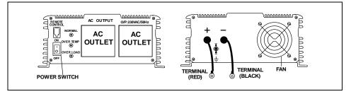
WHEN CONNECTED TO ANY APPLIANCE, BE SURE TO TURN ON INVERTER FIRST. AND THEN, TURN ON THE POWER SWITCH OF THE APPLIANCE.
