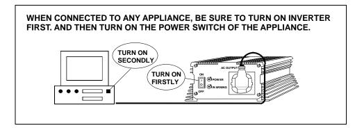
DO NOT USE THE INVERTER BEYOND ITS MAXIMUM OUTPUT POWER. WHEN CONNECTED TO ANY APPLIANCE MAKE SURE THE TOTAL STARTING POWER CAPACITY DOES NOT EXCEED THE MAXIMUM OUTPUT POWER OF THE INVERTER.
