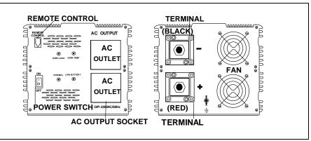
WHEN CONNECTED TO ANY APPLIANCE, BE SURE TO TURN ON INVERTER FIRST. AND THEN, TURN ON THE POWER SWITCH OF THE APPLIANCE.
