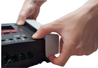
*Fig. 3: Release the cover from the end position (here the right cover)*
