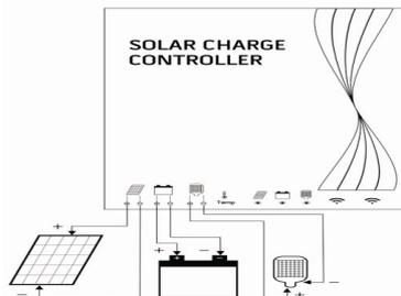
Connection sequence: Please connect the storage battery first, then connect the load, last is the solar panel. Pay attention to the "+" and "-" in case of reverse connection.
