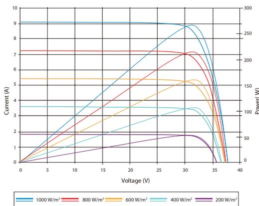
Excellent performance under weak light conditions: at an irradiation intensity of 200 W/m<sup>2</sup> (AM 1.5, 25 °C), **96.5%** or higher of the STC efficiency (1000 W/m<sup>2</sup>) is achieved
